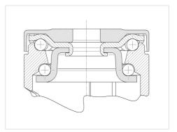
Swivel castor with total lock, tail end of castor, housing and wheels made from high grade synthetic materials, double ball bearing swivel head, bolt hole. Wheel centre made of Polypropylene, Tread: TENTEprene (thermoplastic rubber), grey non-marking, precision ball bearing Hint: These castors are also with grey locking lever available.
