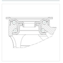
Swivel castor with total lock, tail end of castor, housing made of Polyamide, double ball bearing swivel head, plate fitting. Wheel centre made of Polypropylene, electric conductive, Tread: TENTEprene (thermoplastic rubber), electric conductive, grey non-marking, with threadguards, plain bearing
